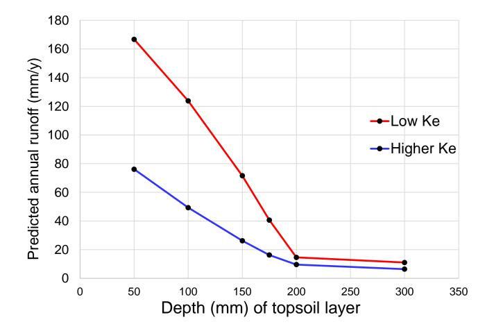
Victorian site, subsoil infiltration rates of 4.8 (low) and 13.2 mm/h (higher)
